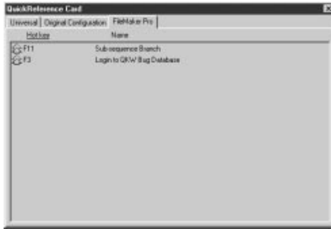
Figure 31: Use the QuickReference Card to help remember your hot keys. In this example, FileMaker Pro is the active program so the Actions scoped to FileMaker appear in the frontmost tab of the QuickReference Card.
