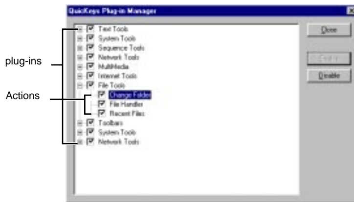
Figure 24: Use the QuicKeys Plug-in Manager to enable or disable plug-ins and Actions.
