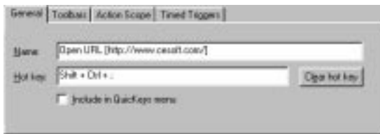
Figure 23: This graphic shows the upper half of the Action Properties dialog where the Clear hot key button is located. To open the Action Properties dialog for editing, double-click the Action you want to edit in the My Actions tab.
